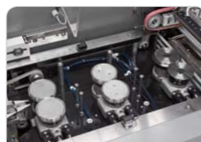
Longitudinal sealing system with tilting rollers
